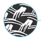
Mutifilament Mesh is a woven fabric where each strand consists of many smaller diameter threads. Multifilament Mesh filters are manufactured in a narrow range of micron ratings using a multistrand weave, and are available in nylon and polyester.
